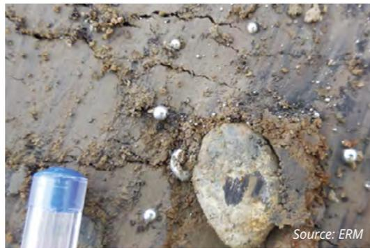
Elemental Hg can collect in features such as subsurface drains, and the foundations, walls, floors and metallic structures surrounding industrial processes can incorporate Hg through adsorption. As a result, the selected site investigation techniques should be tailored to account for non-uniform contaminant distribution (so-called “nugget effect”).
