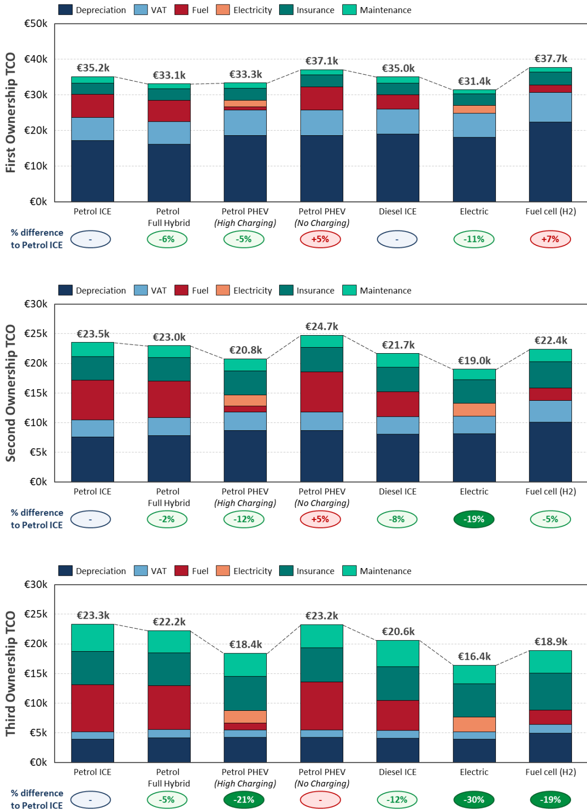
Figure 61: TCOs on a cost component level for different powertrains bought new in 2030
